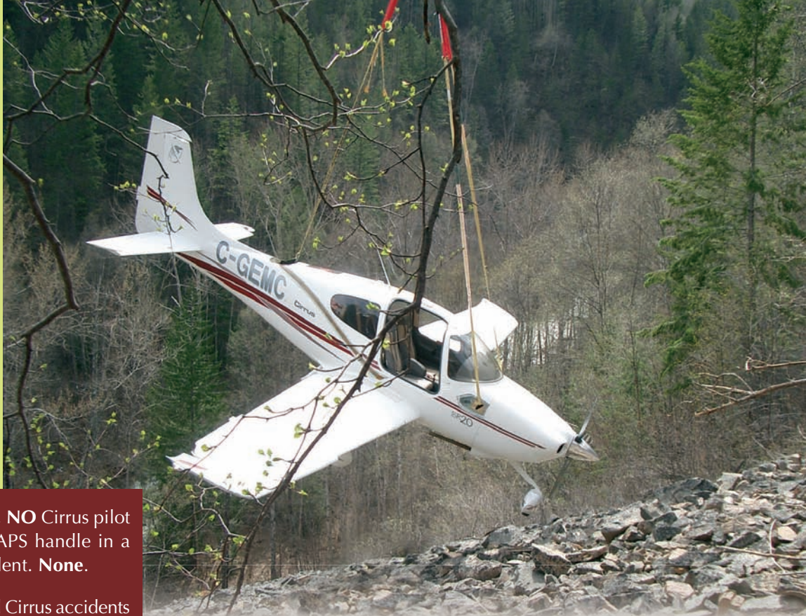
Albert Kolk's SR20 was lifted from the rugged mountains of British Columbia by helicopter using the parachute risers as lifting straps. The plane was repaired and flew again. Other Cirrus pilots have had high-altitude upsets that ended in fatal crashes.
