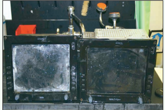
FIGURE 1: Avidyne EXP5000 MFD (left) and PFD (right) after removal from accident airplane N91MB, which had crashed into a retention pond, then transported to the NTSB submerged in fresh water, for preservation, in a cooler. (NTSB photo)
